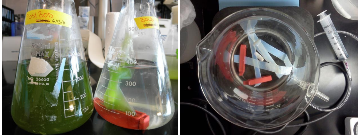
Figure A1. Experimental set ups for preliminary ICARUS tests using dialysis bags of regenerated cellulose and cellulose acetate. Photographs courtesy of Breeyn Greer.
